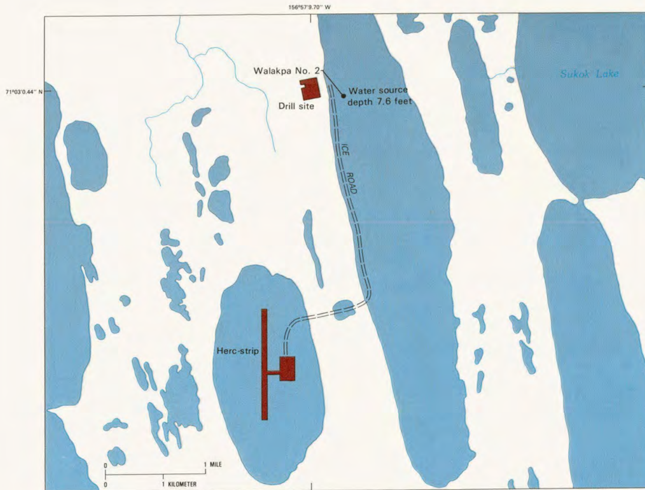
Example of a carefully planned, environmentally sensitive transportation route at the Walakpa No. 2 test well. Instead of a straight road connecting the well to the airstrip, the chosen route avoided the tundra surface as much as possible by taking advantage of every lake, pond, and river along the way.
