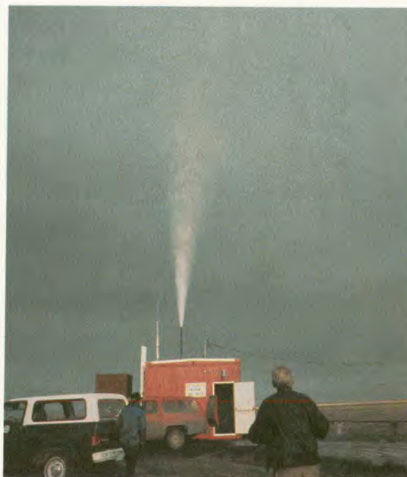
“Blowing” a well. Water vapor produced with the gas freezes out of the slow-moving gas and accumulates in the bottom of the well. To clean out the water, the flow of gas is diverted to the tubing, and the well is opened to the atmosphere. The gas flowing against only atmospheric pressure through the small-diameter tubing attains a high velocity and carries the water to the surface. The water is discharged into the air as vapor, forming a plume. Photograph by Robert Lantz.
