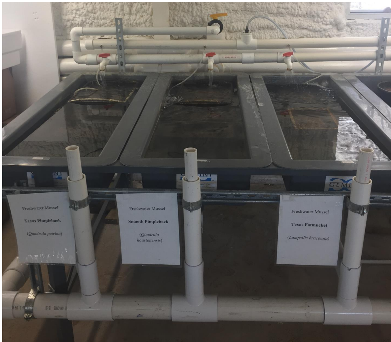
Figure 13. Indoor flow-through raceway system for holding adult freshwater mussels at Inks Dam National Fish Hatchery
