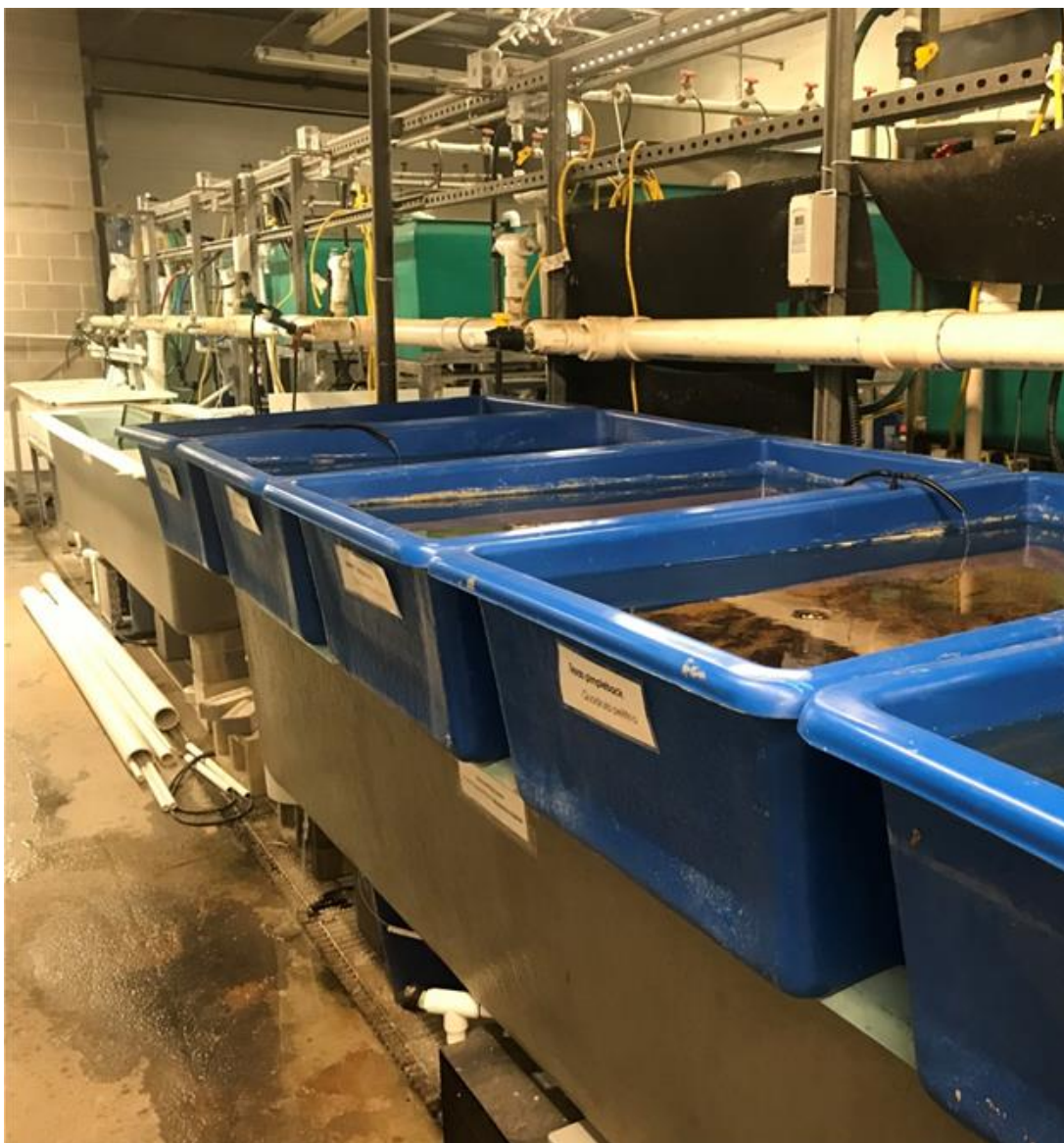
Figure 6: Indoor recirculating systems used for long term holding of adult mussels in 2017.
