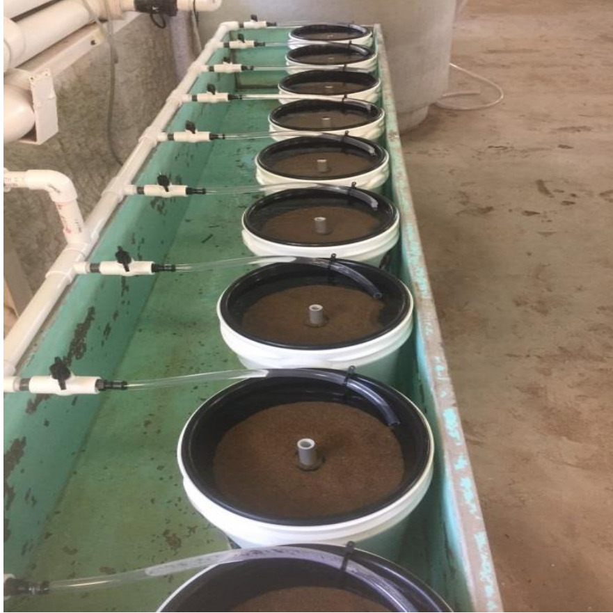
Figure 10. Flow-through juvenile mussel rearing system at IDNFH.
