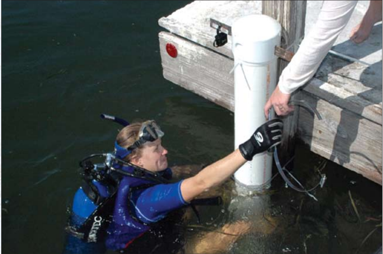
Staff monitors water quality with the use of dataloggers that record continuous data including dissolved oxygen, salinity, temperature, pH and turbidity every thirty minutes.
