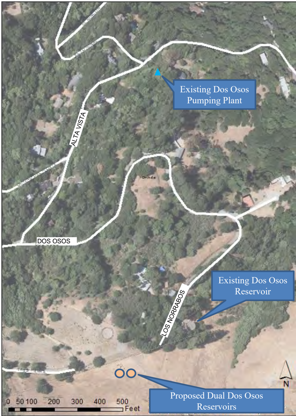
Aerial Photo View of Major Dos Osos Reservoir Replacement Project Components Figure 2.5
