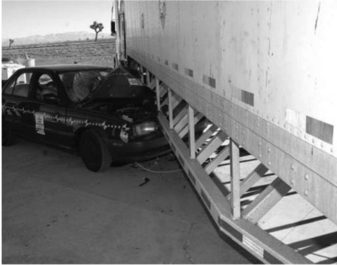
Figure 4 SUG designed and tested by Kumar et al. (2009).
