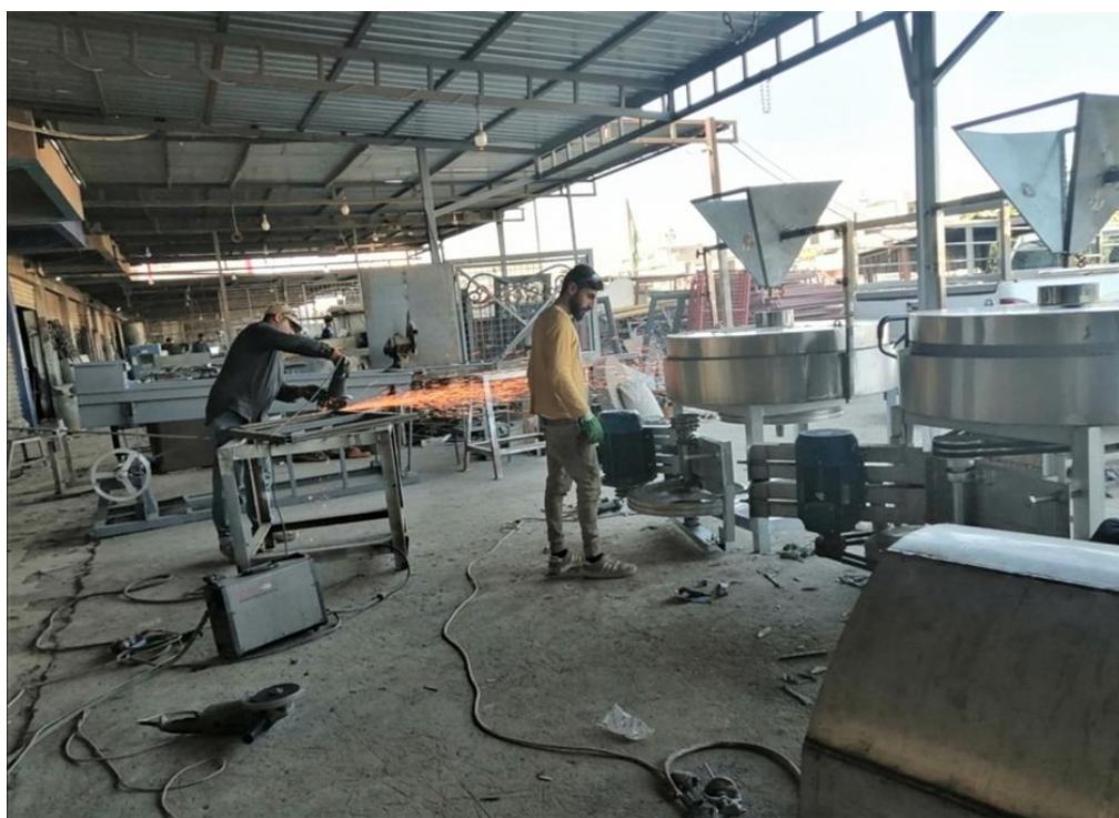
Fabrication by a local company of the sesame seed stone grinder equipment ordered
