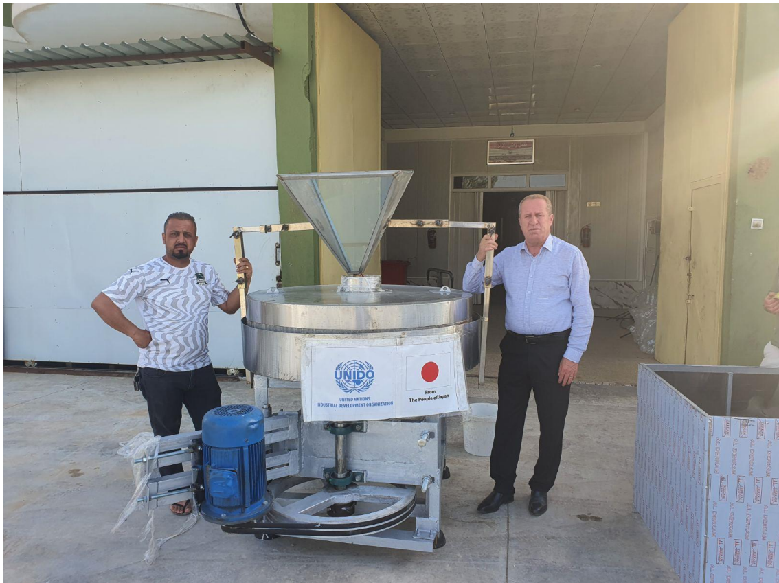
Sesame Seed Stone Mill Grinder (locally fabricated) Handed Over to an SME Tahini Factory
