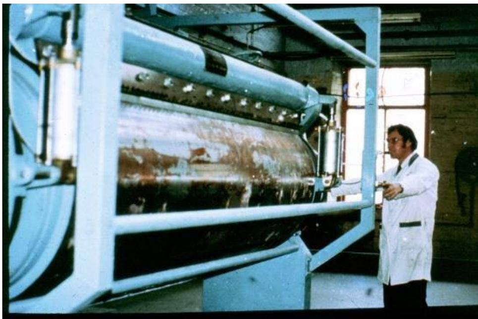
Here is the commercial version of the rotary drum dryer at Pedigree Petfoods being installed at the Thomas's factory at Shelf, near
