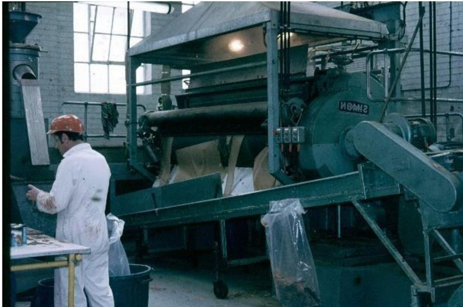
A conveyor belt was also installed to move the flakes from the roller and cutter to the packing area.
