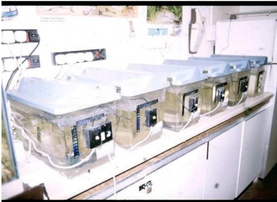
This was a novel heater where a heating element was buried in a flat plastic plate and an electronic control unit, sealed in resin,
