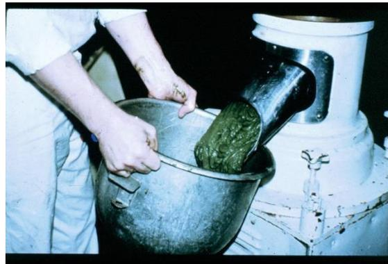
Foods were blended in a Hobart Bowl and the mixture added to the emulsifier, which reduced the mix to a flowing paste.
