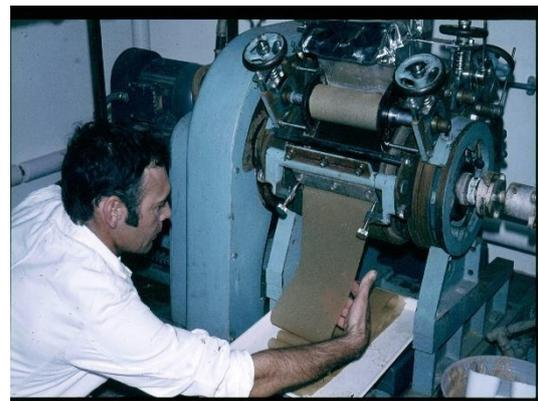
The food pastes were poured into the funnel and from there pumped at a controlled rate onto the steamheated roller drier. This flashcooked the proteins to give a paperlike texture, just as occurred with the frying pan and wallpaper
