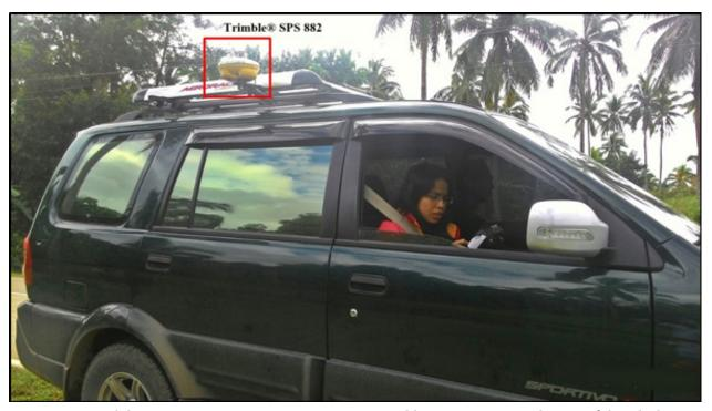
Figure 44 Validation points acquisition survey set-up: A Trimble® SPS 882, mounted on top of the vehicle
