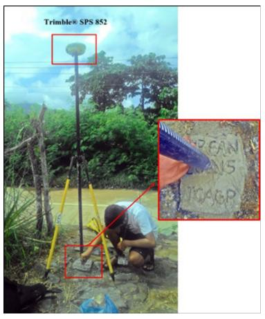
Figure 39 GNSS receiver set-up, Trimble® SPS 882, at UP-GAN, located on top of a riprap near Gangao Bridge, along Central Nautical Highway, Brgy. Gangao, Baleno, Masbate
