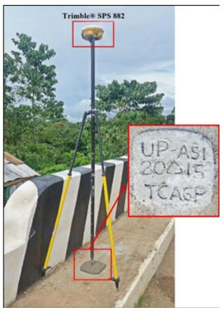
Figure 38 GNSS receiver set-up, Trimble® SPS 882, at UP-ASI, located at Asid Bridge, along Central Nautical Highway, Brgy. Asid, Masbate City
