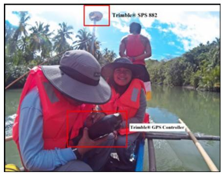
Figure 46 Bathymetric survey set-up using OHMEX™ single beam echo sounder and amounted with a Trimble® SPS 887
