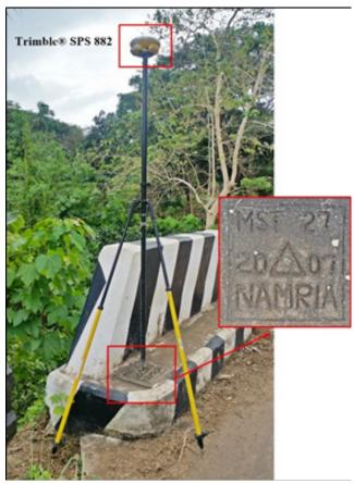
Figure 36. GNSS receiver, Trimble® SPS 882, at SE-85, located at the approach of the Llorente Bridge in Barangay 11, Municipality of Llorente, Eastern Samar
