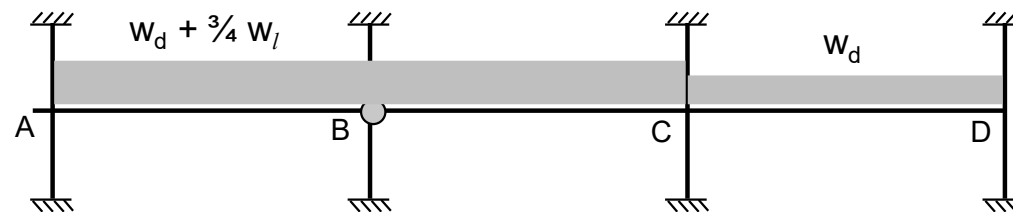
(5) Loading pattern for negative design moment at support B'
