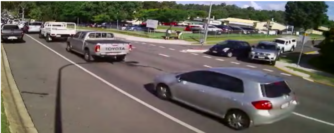
Figure 2-15 Motorist attempting to pass queued right turn vehicle
