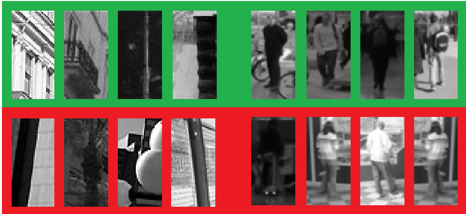
Figure 6.4: Examples of true and false classifications from the INRIA dataset. We can see that the network is overexcited over high contrast vertical edges. This can be counteracted by expanding training examples of this type in the training set.
