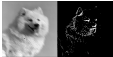
Figure 3.9: Visualizing activations - the input image(left) and the activations of a trained convolutional filter(right)
