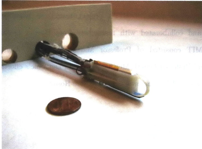
Figure 4: SQUISHbot traversing through hole using its prismatic joint & anisotropic footpads.
