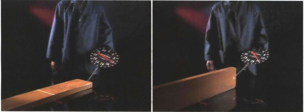
Figure 9: A scale pulling a plank demonstrates that frictional force is approximately contact area independent. Image reproduced from [10].
