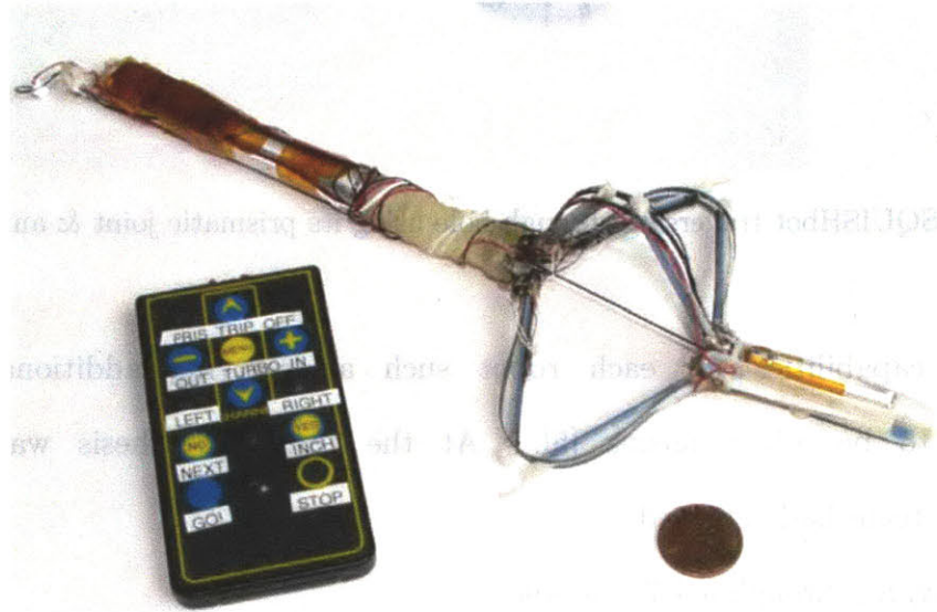
Figure 3: SQUISHbot with active-fluid joints. String is attached to the spooler motor.
