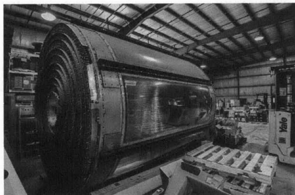
This central tracking chamber fit in the center of the Collider Detector at Fermilab. Its job was to trace the debris from particle collisions (Brian Nord, Fermilab).
