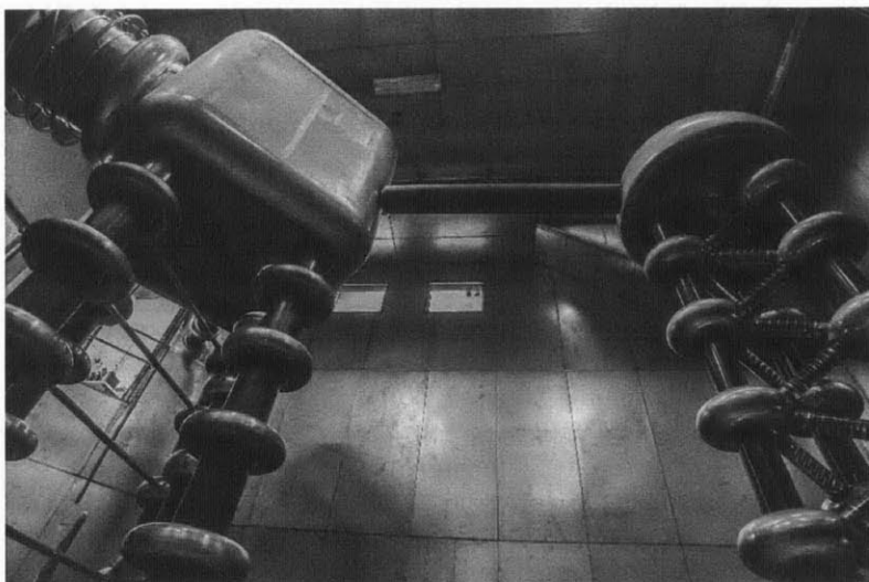
From below, the towering Cockcroft Walton looks like something out of science fiction. Hydrogen atoms used to shoot out of the Faraday cage on the left, through a tube and into the lab's accelerator chain (Brian Nord, Fermilab).
