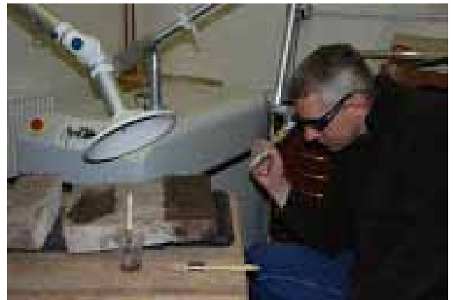
Figure 99: Laser treatment to remove soiling from a carved stone in the St Vigens Museum. Crown Copyright: Historic Environment Scotland
