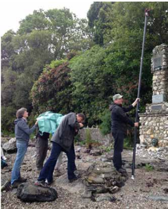
Figure 78: Using a 'magic pole' telescopic rod to photograph hard-to-reach sections of a WWI memorial. Ensuring complete and overlapping coverage of sites or objects is essential for photogrammetric modelling. Colintraive, Argyll and Bute. © CC-NC-BY the ACCORD project
