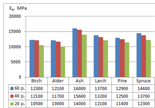
Figure 4 – Dynamics of change of the initial modulus of elasticity of solid wood of deciduous and coniferous breeds at different ages
