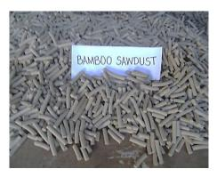
Pellets from bamboo sawdust produced using the FPRDI pelletizing machine.
