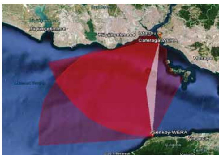
Figure 13. Proposed HF-radar deployment to cover Bosphorus outflow (red patch is where full current vectors can be recovered).
