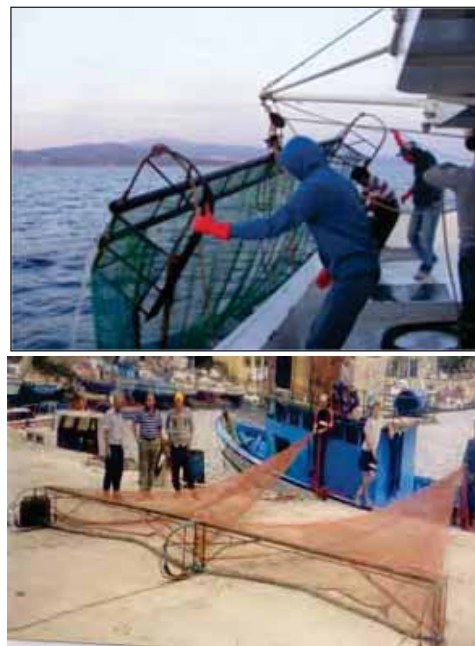
Figure 2. Single beam trawl and twin beam trawl used in the Sea of Marmara (Zengin et al. 2004, İşmen et al. 2015) A. Single beam trawl, B. Twin beam trawl.
