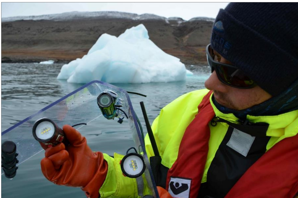
Figure 9. Video footage was recorded using a Paralenz underwatercamera supplemented with LED lamps
