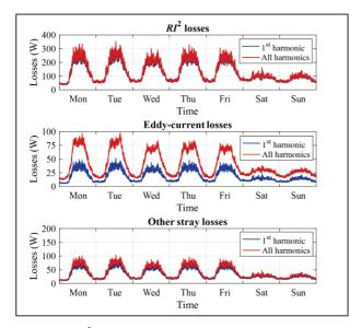
Figure 3.  $RI^2$ , eddy-current and total stray losses with and without considering real measured harmonics for one week
