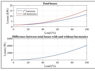
Figure 2. Total losses with and without considering harmonics depending on transformer load
