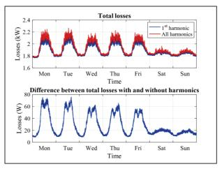
Figure 4. Total losses with and without considering real measured harmonics for one week
