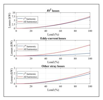
Figure 1. *RI*<sup>2</sup>, eddy-current and total stray losses with and without considering harmonics depending on transformer load
