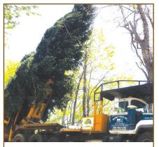
The truck's massive hydraulic cylinders raise the tree above the hole. A second set of cylinders will lower the spruce into the planting pit. The tree weighs 17,000 pounds!
