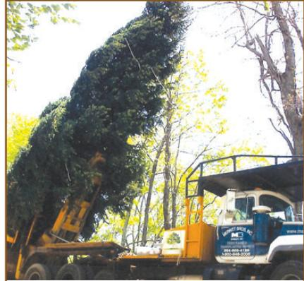
*The truck's massive hydraulic cylinders raise the tree above the hole. A second set of cylinders will lower the spruce into the planting pit. The tree weighs 17,000 pounds!*
