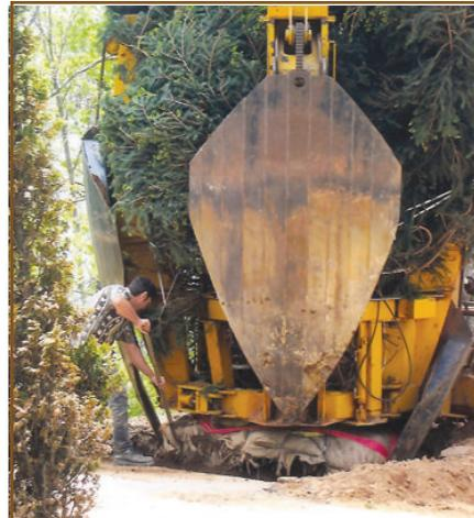
*A worker begins to backfill the hole after the tree spade's huge blades have been retracted, leaving the rootball properly seated in the hole. The machine's yellow heavy metal frame stabilizes the tree during installation.*
