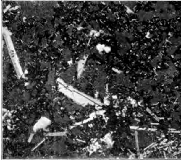
Fig. 1. Trachyte with porous groundmass with much glass and numerous small lath-shaped crystals of orthoclase. Enlarged \times 40 .
