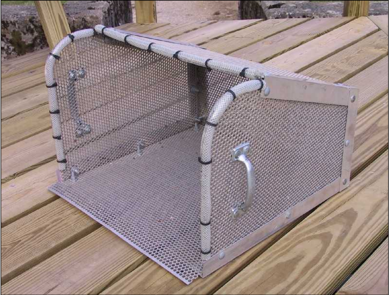
Figure 5. The Ferraro streambed sampler. This sampler is made with perforated aluminum and was designed to hold all substrate excavated from a 0.25 m 2 quadrat.
