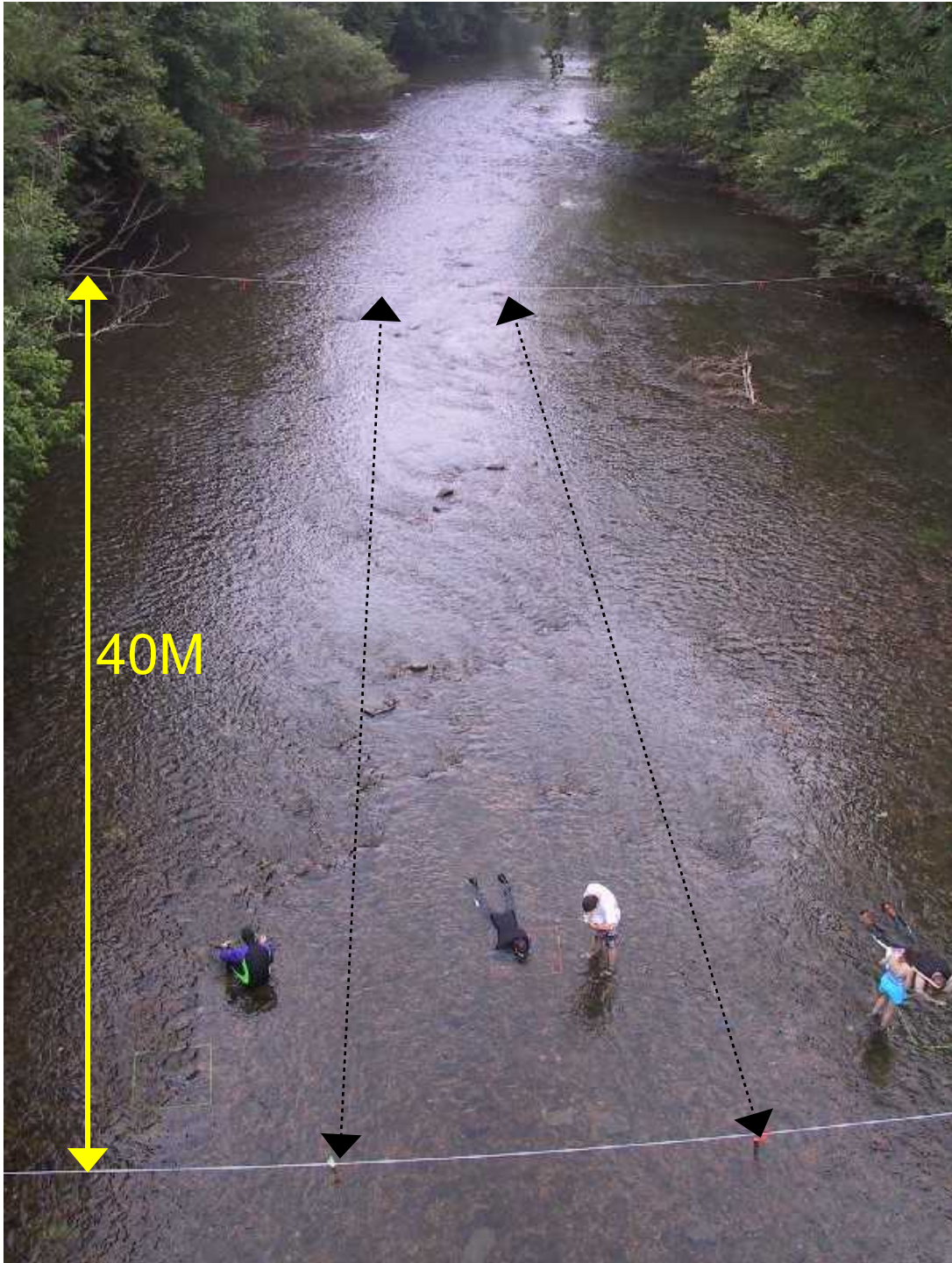
Figure 3. Overhead view of the 833 bridge site. Ropes are stretched every 40 meters with flags to delineate lanes and serve as a visual guide. Black lines show one lane.
