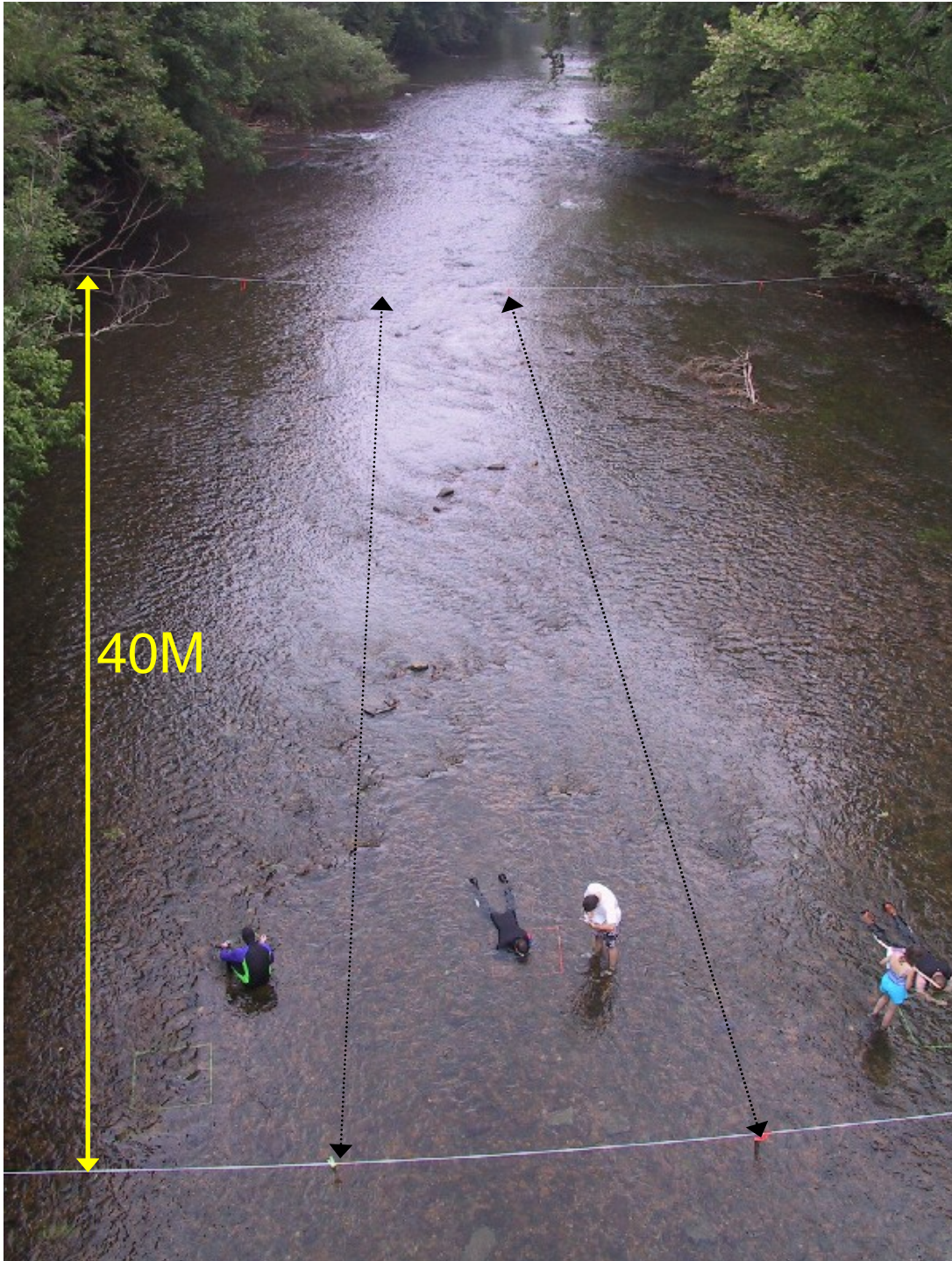
Figure 4. Overhead view of a survey site. Ropes are stretched every 40 meters with flags every 5 meters to delineate lanes and serve as a visual guide. Black lines show one lane.
