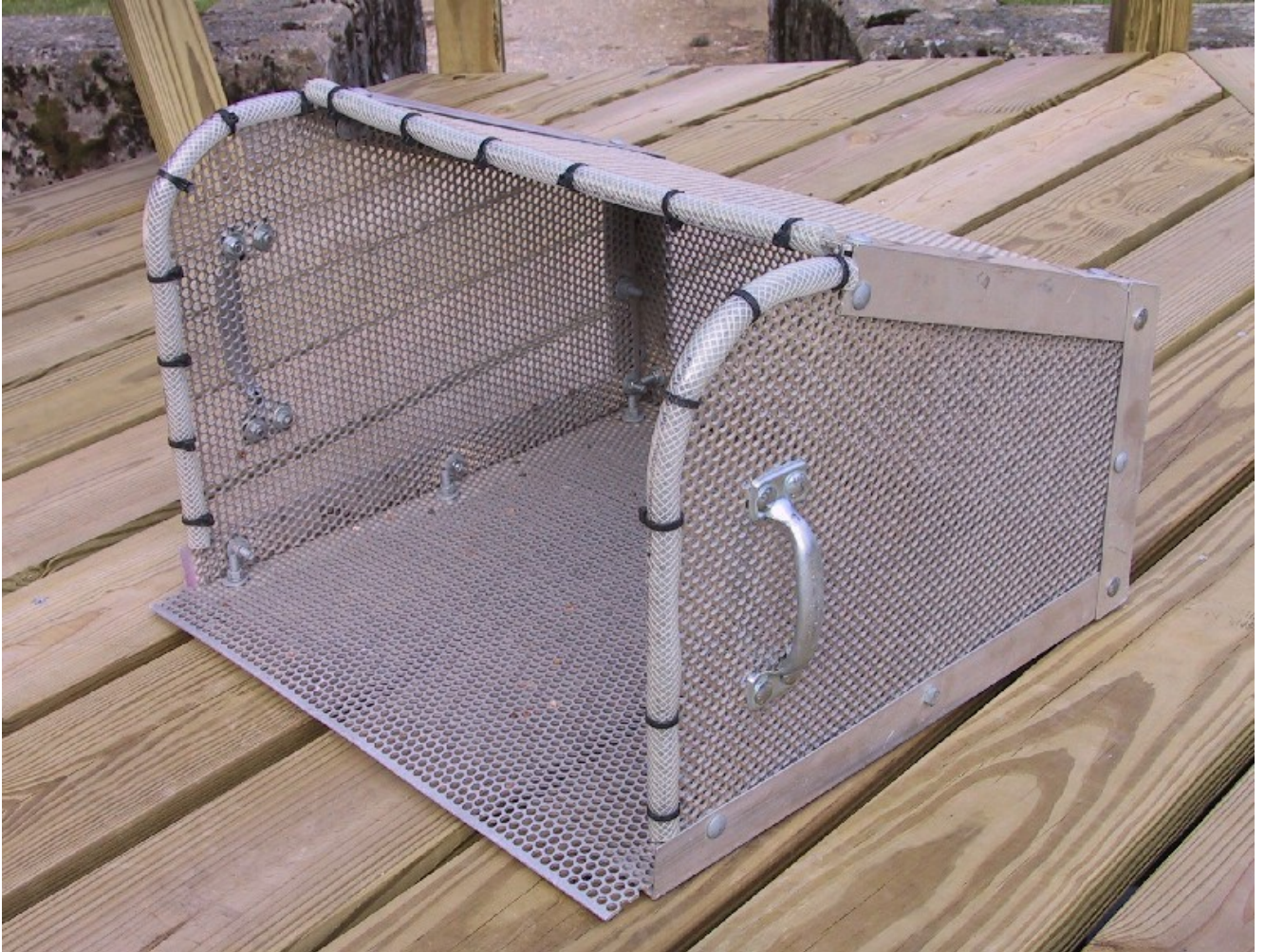
Figure 6. The Ferraro streambed sampler. This sampler is made with perforated aluminum and was designed to hold all substrate excavated from a 0.25 m 2 quadrat.
