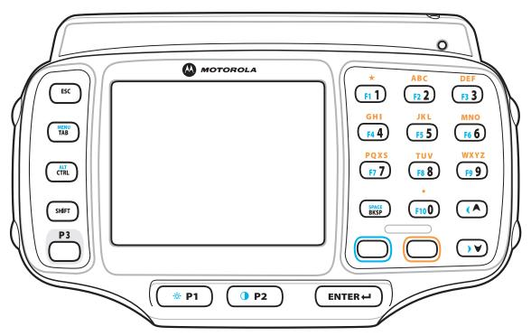
Figure 2-5 Triple-tap Alphanumeric Keypad
