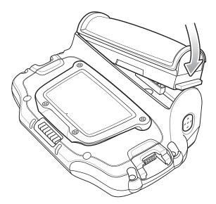
Figure 1-7 Installing the Main Battery
