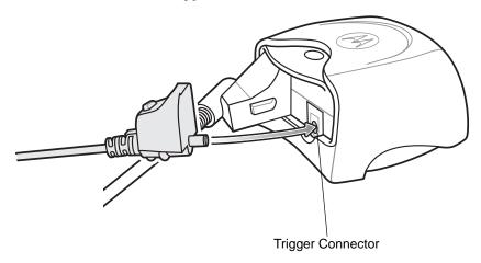
Figure 3-8 Connecting Trigger Cable to RS309
