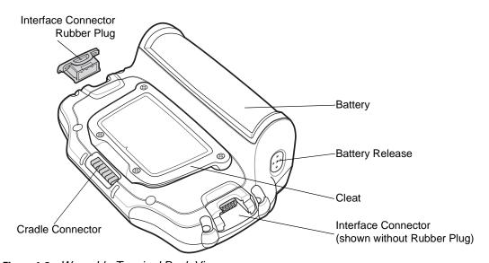
Figure 1-3 Wearable Terminal Back View
