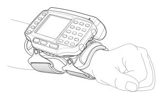
Figure 1-11 Wearable Terminal and Wrist Mount
