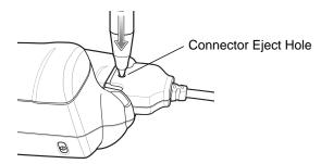
Figure 3-18 Disconnecting Connector with Shroud
