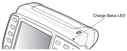
Figure 2-2 Wearable Terminal LED Indicators
