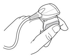
Figure 3-6 Place the RS409 on Index Finger
