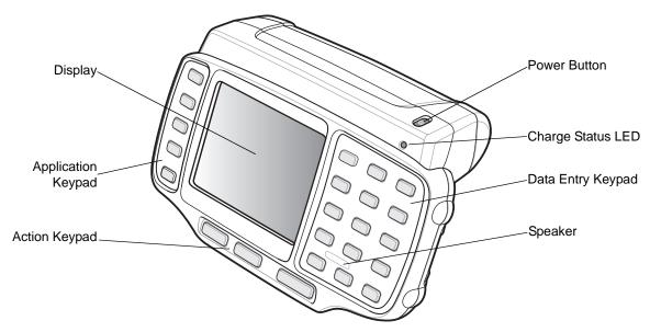
Figure 1-1 WT4070/90 Wearable Terminal Front View
