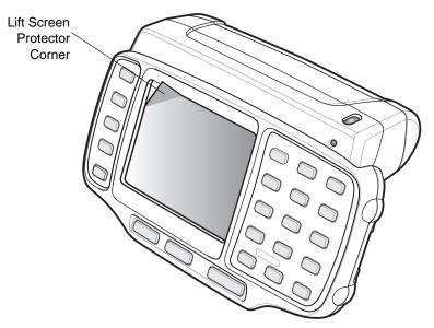
Figure 4-2 Removing the Screen Protector
