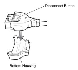
Figure 3-16 Installing Bottom Housing
