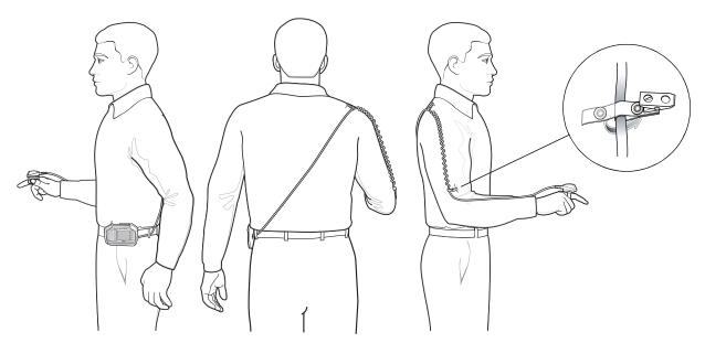
Figure 1-16 Routing RS409 Scanner Cable from Hip to Hand
