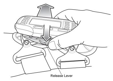
Figure 1-12 Wearable Terminal Removal
