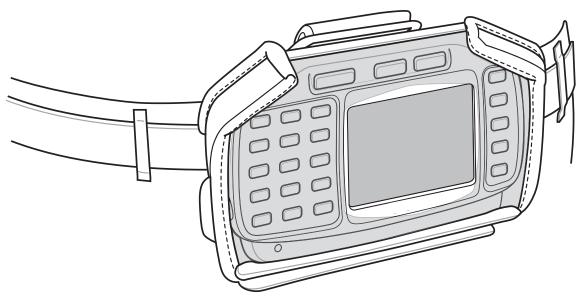
Figure 1-15 Hip Mount on Belt
