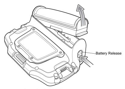
Figure 1-8 Removing the Main Battery
