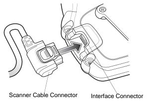
Figure 3-4 Connecting RS409 to Wearable Terminal
