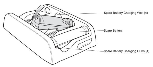
Figure 3-3 Four Slot Spare Battery Charger
