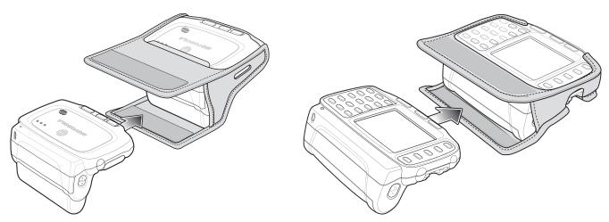
Figure 3-11 Insert Wearable Terminal into Freezer Pouch
