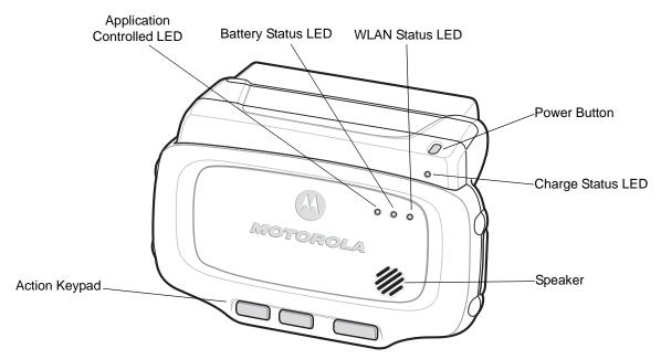
Figure 1-2 Voice Only WT4090 Wearable Terminal Front View
