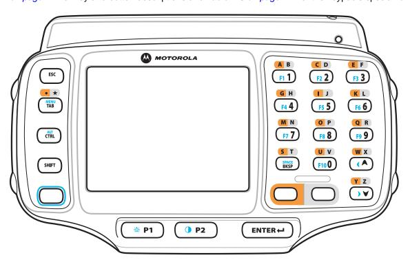
Figure 2-4 Two-color Alphanumeric Keypad
