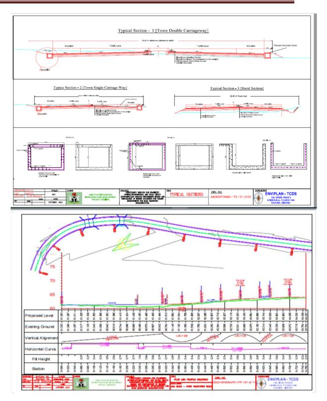
Figure 3.5: Road profile of the Aba Road project
