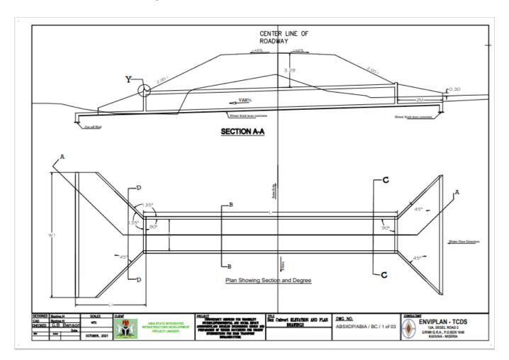
Figure 3.2 Box Culvert In Let And Out Let 01
