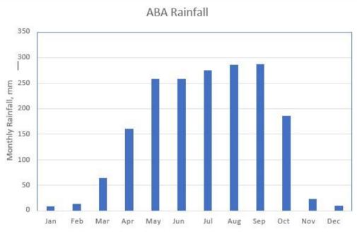
Figure 4.3: Long Term Rainfall station at Aba Station
