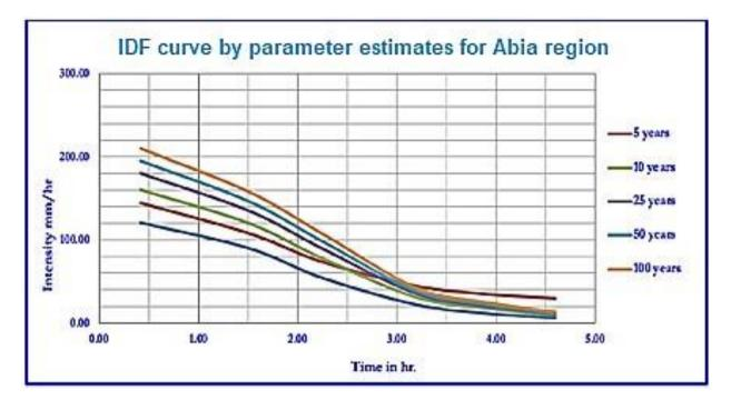
Figure 4.4: Rainfall Intensity-Duration Frequency Curve for Abia State
