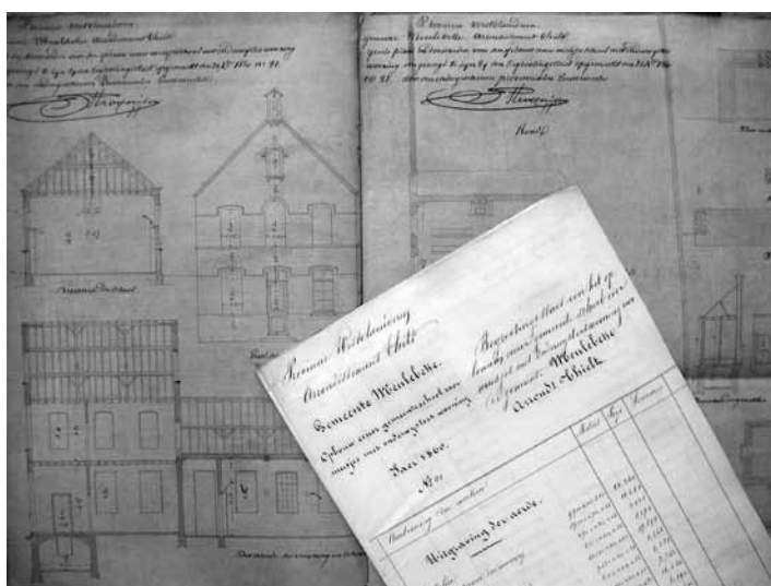
Figure 2. Plan and building estimate by Pierre Nicolas Croquison for the construction of a municipal primary school in the village of Meulebeke, 1860. The building estimate is handwritten, following a template systematically used by Croquison for all his designs. (source: Bruges, State Archives, Archive Provincie West-Vlaanderen, 4e afdeling, 232)
