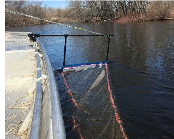
Figure 2: Neuston net used to sample larval Lake Whitefish in the four major Green Bay tributaries
