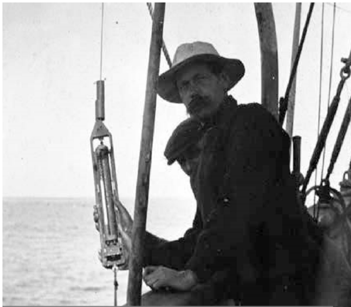
Fig. 23: Dannevig and crewman demonstrating the Ekman reversing bottle on a voyage from Melbourne to Eden. Photo by Captain J.K. Davis. Courtesy State Library of Victoria, John King Davis Collection.
