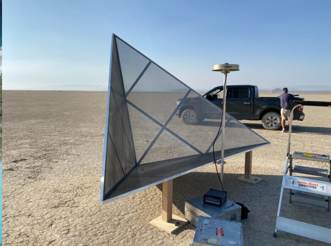
2.8 m L-band trihedral reflectors for NISAR
