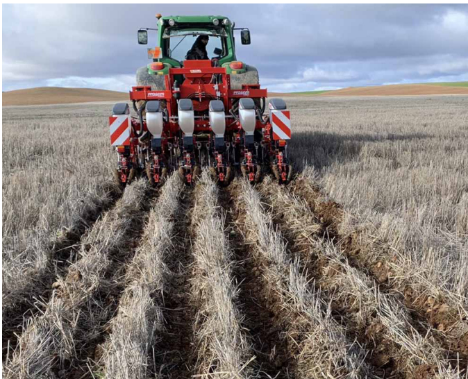
Figure 2.3. Strip seeding machine. Source: Empresa Agraria.
