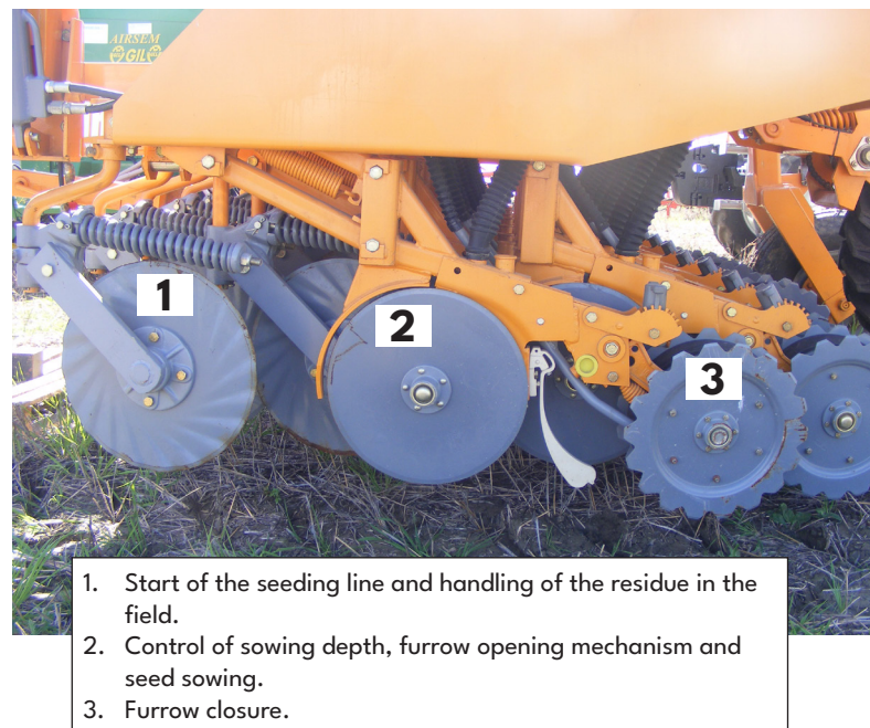
Figure 2.6. Sowing unit of a direct sowing seeder. Source: ECAF.
