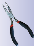
Pliers to break out cable guides
