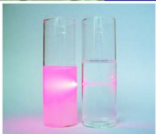
▲ Figure 11.20 Tyndall effect in the laboratory. The glass on the left contains a colloidal suspension; that on the right contains a solution. The path of the beam through the colloidal suspension is visible because the light is scattered by the colloidal particles. Light is not scattered by the individual solute molecules in the solution.
