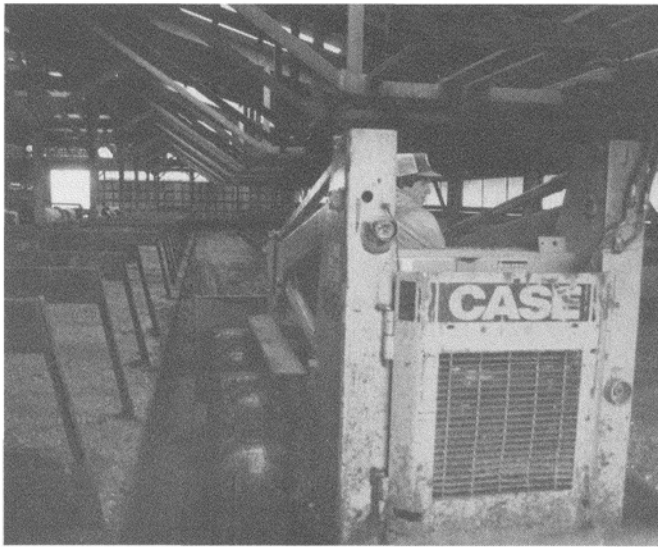
Three steps in converting manure to methane gas: Above, a worker drives a front-end loader that pushes waste along a barn floor and into a hopper at the far end. Manure is shoveled
