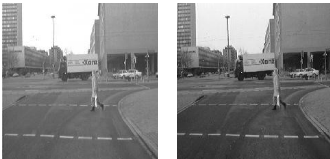
Figure 5.3: The street image pair used as test data for the gradient-based stereo method. The image pair is challenging in that it contains large untextured areas and global intensity differences due to different camera characteristics. The images are displayed in reverse order to allow free fusing.
