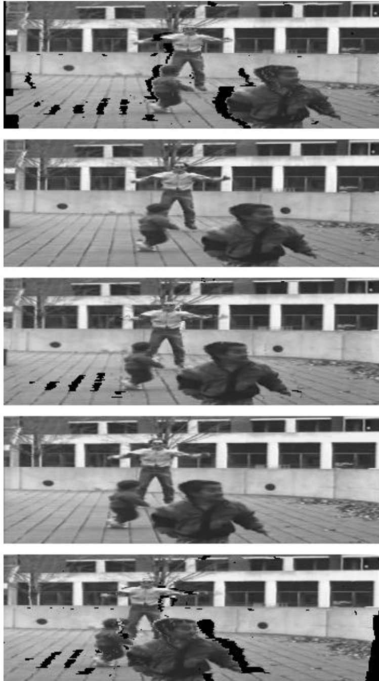
Figure 3.5: Synthesized views for the kids image pair from different positions along the baseline. The second and fourth row contain the original images. The holes are shown in black.
