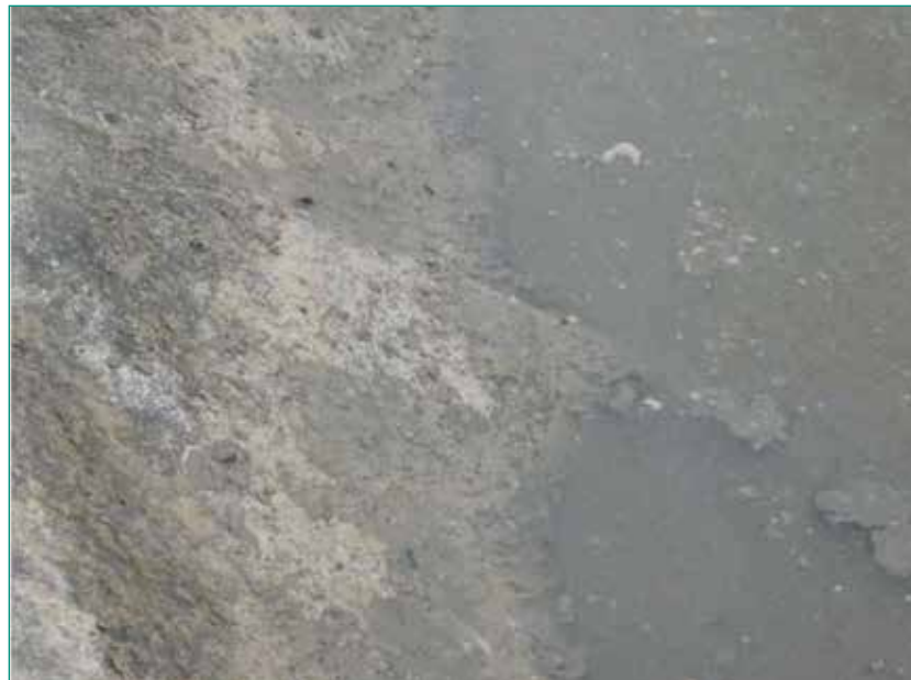
Fig. 1: Initial evaluation of the wastewater shows water that is dark in color with sludge and some black solids floating on the surface.
