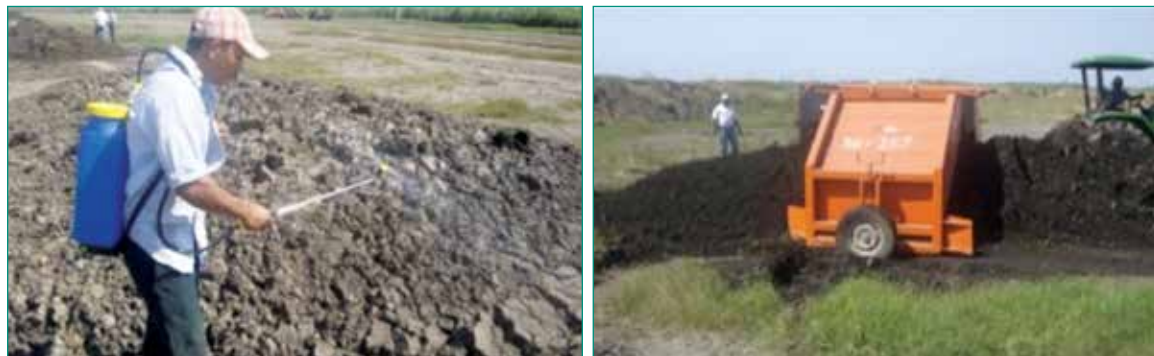
Fig. 8 & 9: Each dose is sprayed on the row before the aerating tractor turns the row to mix, allow gases to escape, and oxygenate the cultures.
