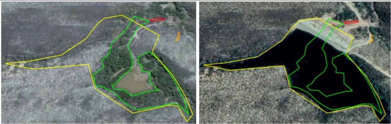
Figure 4: Enlarged dam shown pre- and post-construction with impacted aquatic habitat overlaid. Green = riparian vegetation, yellow = enlarged dam footprint, Orange = sand discard in wetland, and, Red = rock discard in drainage line.
