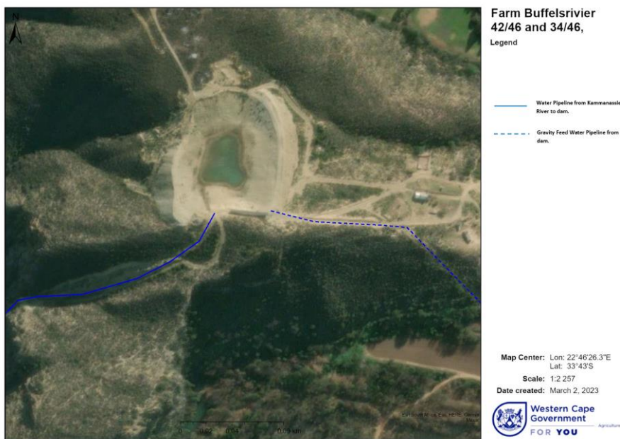
Figure 9: Water Pipelines for Kop Dam.
