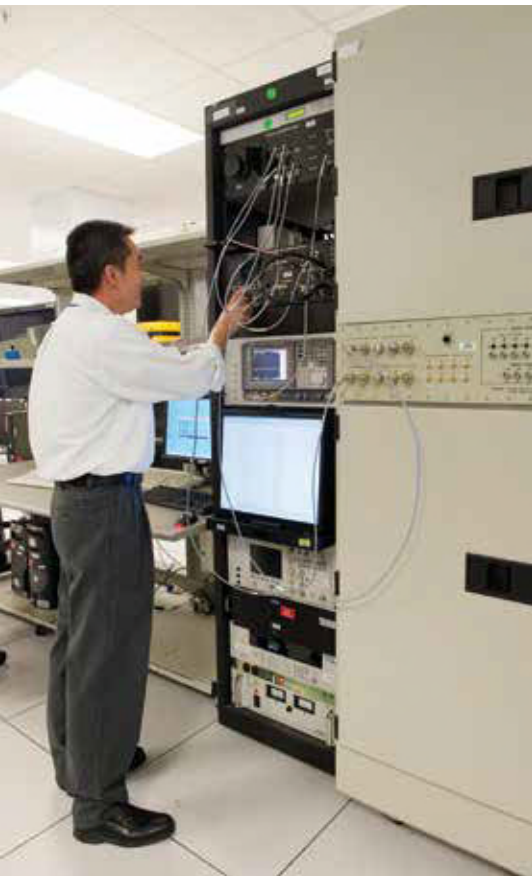
ARAT assistant project lead prepares to test the AN/APR-39B(V)2 system with the AMES II RF Simulator.
