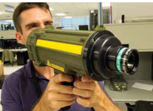
ARAT hardware technician utilizing the Baraga test set to trigger CMWS.
