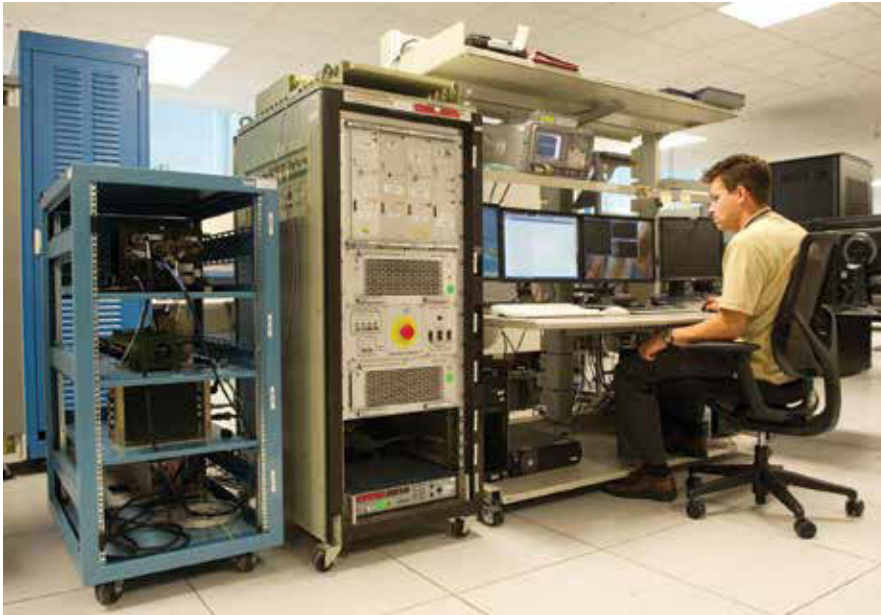
ARAT Engineer testing the RFIS system with the Micro AMES RF Simulator.
