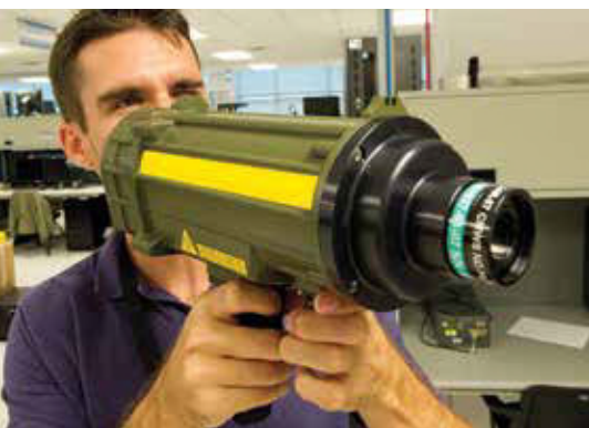
ARAT hardware technician utilizing the Baraga test set to trigger CMWS.
