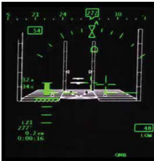
Air Soldier System 3D Degraded Visual Environment (DVE) flight symbology, as displayed to the aviator through a Helmet Mounted Display (HMD) during the July 2013 Crew Station Working Group at Redstone Arsenal, AL.
