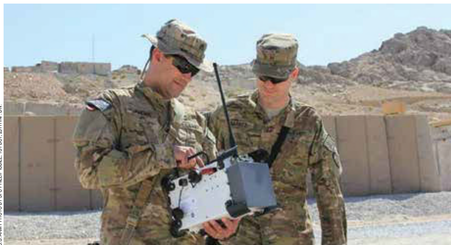
WO1 George A. Warner and SSG Sean E. Adkins initialize the Universal Test Set to ensure EW equipment is operating at the proper frequencies.
