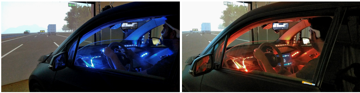
Figure 4.2: A driver in our simulator study, wearing the EEG and heart rate sensors during the blue (left) and orange (right) ambient lighting conditions. The sensors were used to detect the driver's emotions while the ambient light was used to influence driving behaviour. Both light colours improved driving performance compared to a baseline ride due to their warning (orange) and calming (blue) effects.
