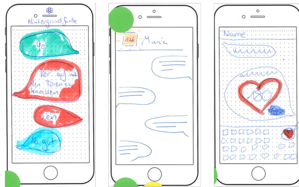
Figure 5.1: The three top-voted concept designs from the user design session: (A) The first design uses colored chat bubbles, where color varies depending on the heart rate of the message sender at the time of message sensing. (B) In the second design, a colored, continuously blinking shape in the chat header is shown. The color refers to the heart rate of the chat partner. (C) In the third design, a button is added to the keyboard for explicitly sending the current heart rate while chatting. The heart rate is shown in a separate message.
