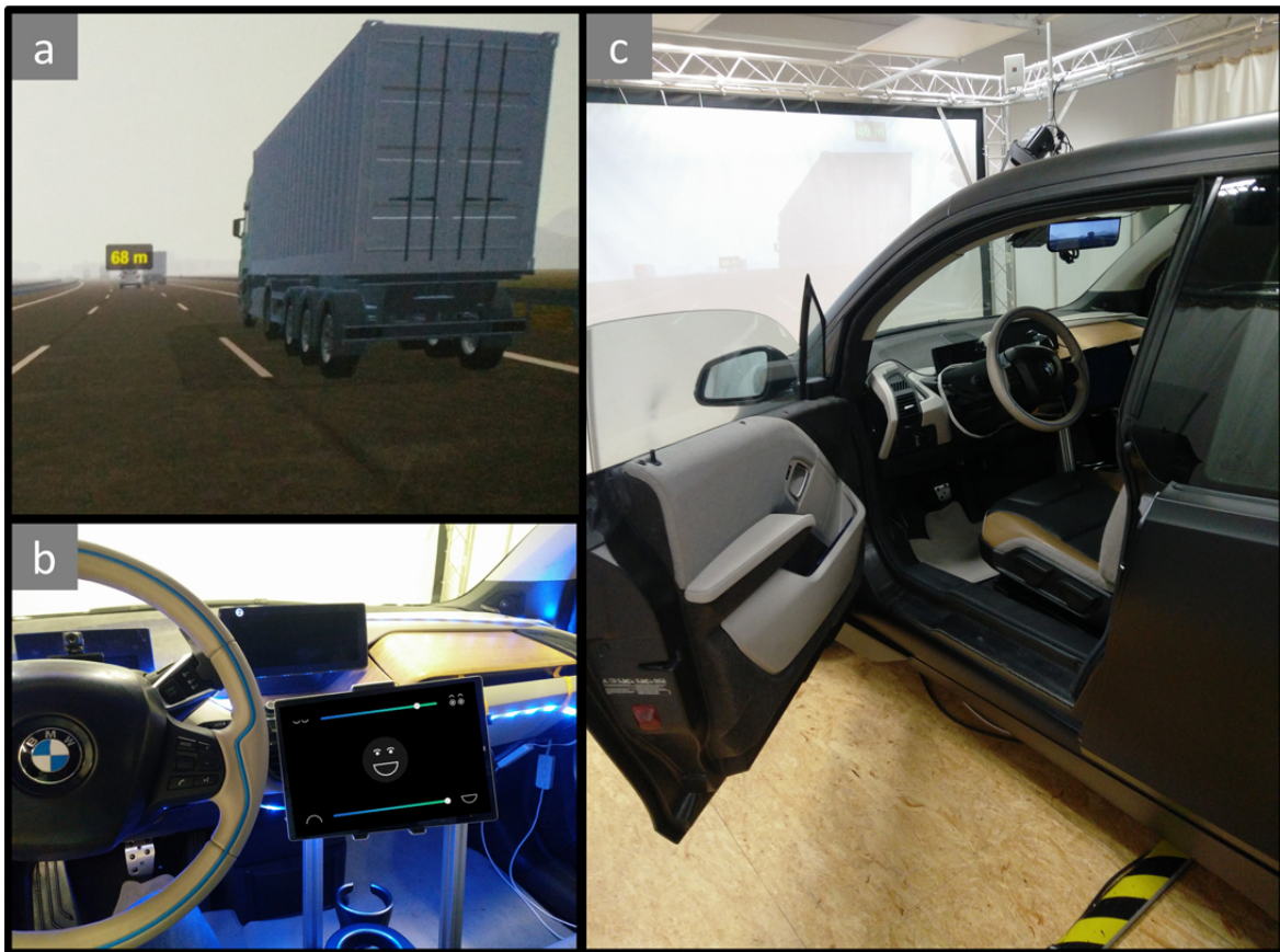
Figure 4.3: Three images showing the simulator study setup: (A) The projected driving scenario during an overtake. The distance to the followed vehicle is shown in yellow (B) The inner dashboard of the car showing the ambient lighting LEDs around the wheel and along the passenger side. On the right, the tablet is shown depicting the continuous SAM scale developed for the experiment. (C) The driving simulator showing the stationary car and the projected driving scenario.
