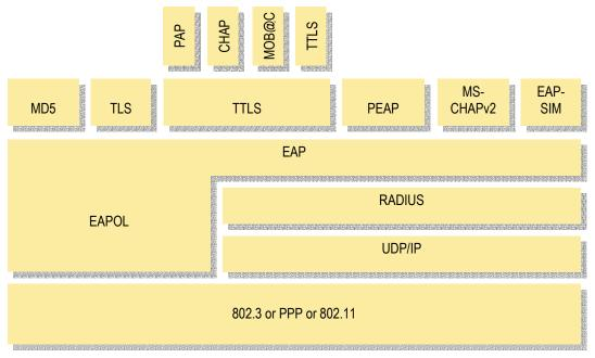
Figure 2: EAP can support various forms of authentication mechanisms
