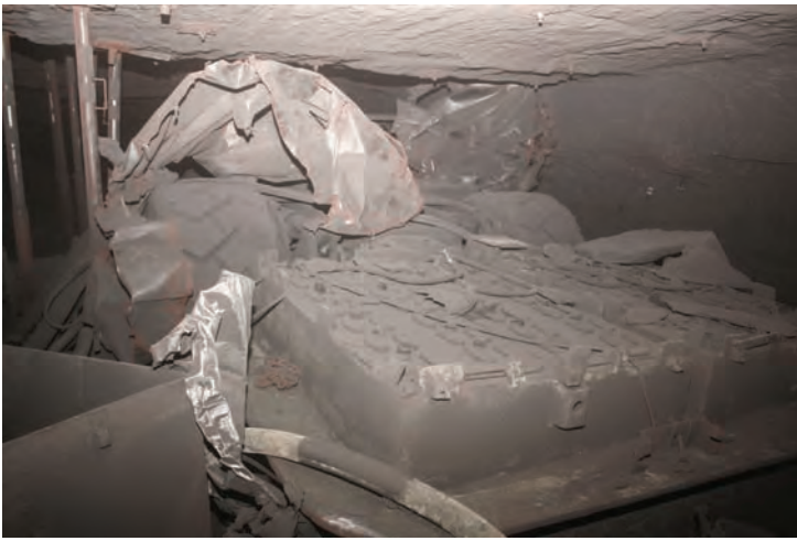
Photo 7. Shield hauler with a steel ventilation door wrapped around the top, found at Headgate 22.
