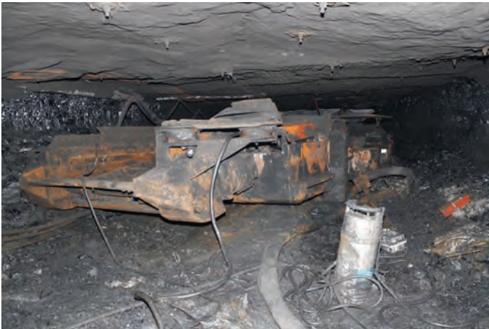
Photo 3. A shuttle car inby the belt dump point in the Tailgate 22 Section shows evidence of the flames and forces of the explosion.
