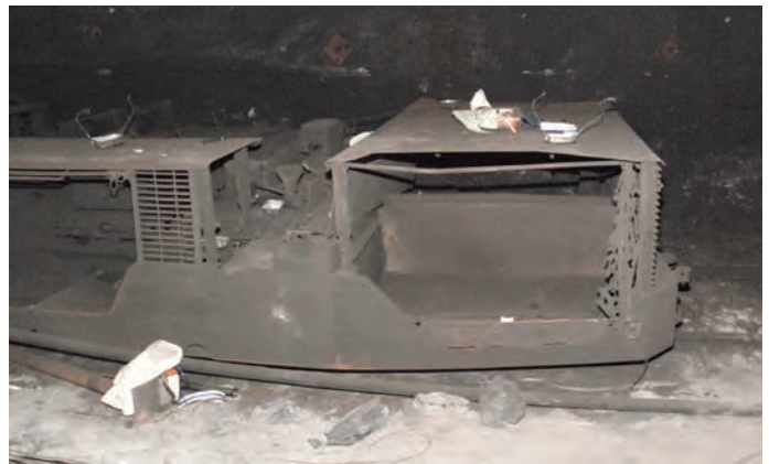
Deployed SCSRs on top of mantrip and on ground at 1 North 21 Longwall track.
