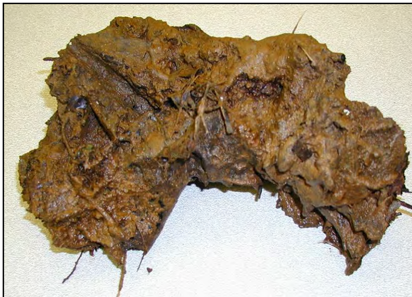
Figure 4. A leaf pack cemented by \text{CaCO}_3 and ferrous oxide. This piece was broken off a larger debris dam in a headwater stream in Martin Co. affected by surface mining. The conductivity was 2350 \mu\text{S}/\text{cm} and the pH was 9.13 S.U.
