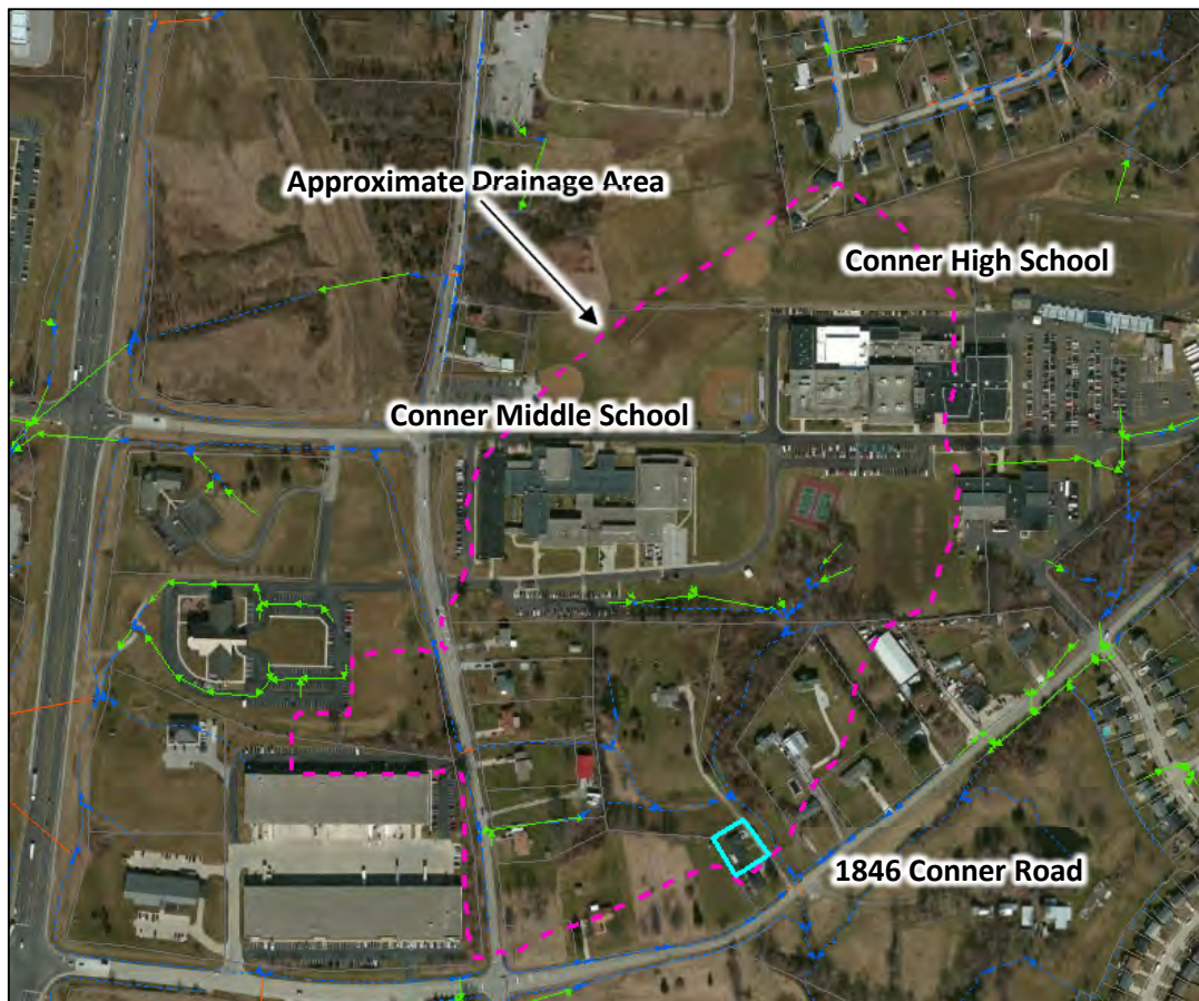
Figure 6-4 – Aerial photo of the 1846 Connor Road property where flooding issues were discussed at the February 4, 2014 Fiscal Court Meeting. The small upstream catchment area includes Connor Middle School, which appears to have inadequate stormwater controls to protect against downstream flooding and stream erosion. As opposed to strictly focusing on increasing the size of the downstream culvert, public funding could be invested in volume-based stormwater controls to solve the root cause of the problem provide numerous benefits to downstream property owners and the health of Gunpowder Creek.
