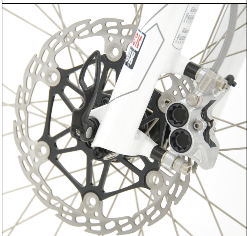
ABOVE. The awesome Hope M4 calliper and 183mm floating rotor.
