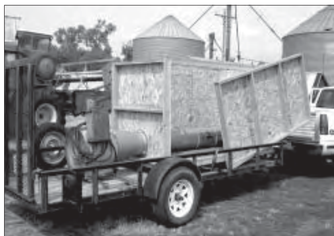
Plywood seed drying box connected to a grain drying fan.
