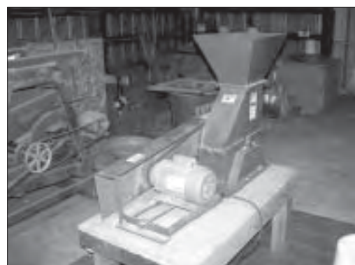
Speed King Hammermill model 615.
