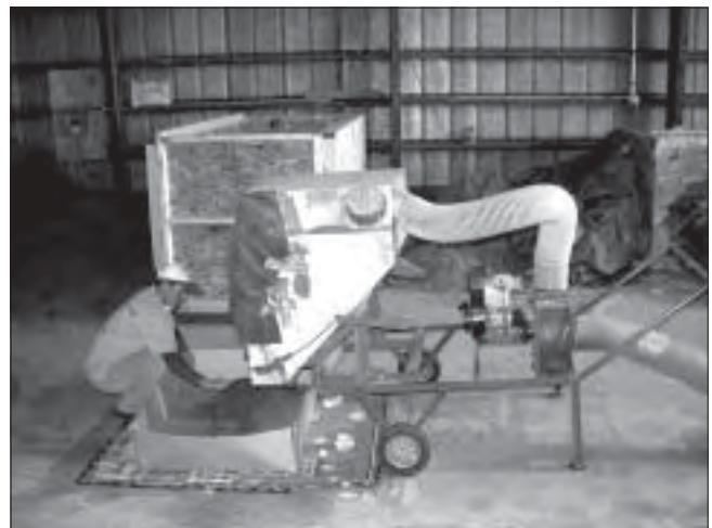
Homemade hammermill consisting of a modified heavy-duty Grasshopper lawn mower conveyor fan run by a gas engine.
