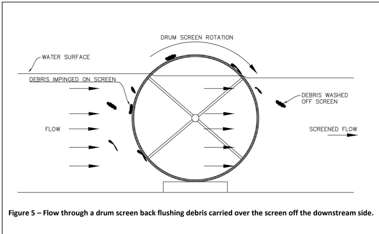
**Figure 5 – Flow through a drum screen back flushing debris carried over the screen off the downstream side.**
