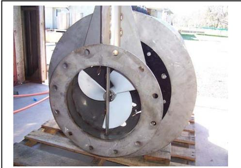
**Screen with propeller drive for rotating the screen cylinder past brush during cleaning.**
