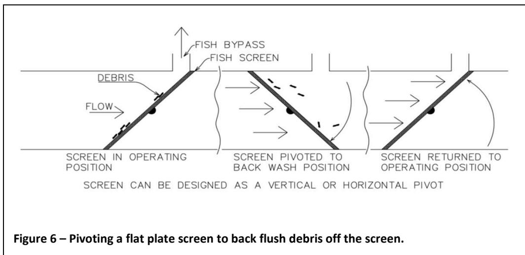
**Figure 6 – Pivoting a flat plate screen to back flush debris off the screen.**
