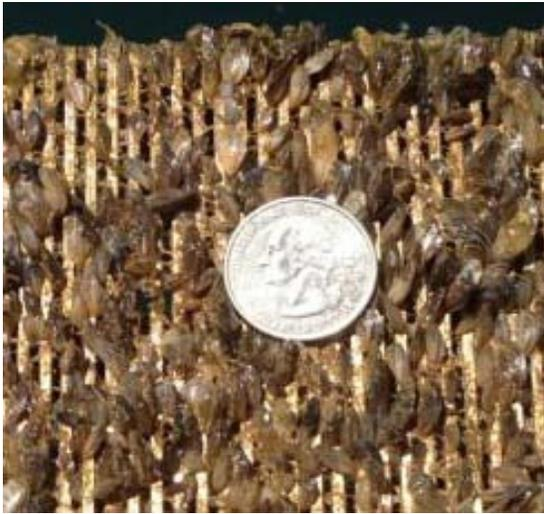
**Figure 10 - View of Quagga mussels and algae on the front face of wedge-wire screen after 3 months without cleaning.**
