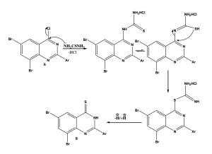
Figure 3: the mechanistic process via which compound 8 is created.
