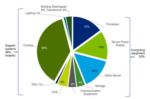
Figure 27: Average distribution of power consumption in a data centre in 2010 (Source: Emerson Power)<sup>30</sup>
