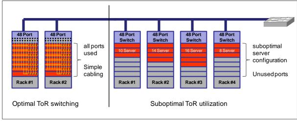
Figure 25: Top-of-Rack switching
