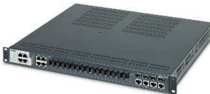
8 RJ45-Ports, 4 Gigabit-Combo-Ports (SFP oder RJ45) und 16 LWL-Ports (Singlemode)
