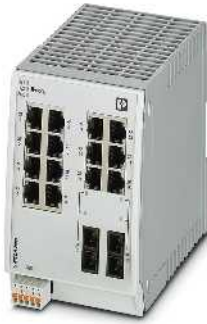
14 RJ45-Ports und 2 LWL-Ports (Multimode)
