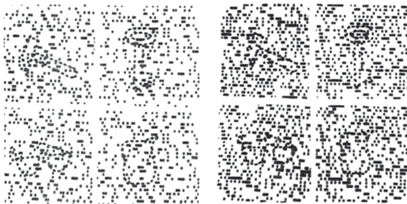
FIGURE 2.1 “Noisy” pictures of the objects. Probability of background black squares is p = 0.25 on the left and p = 0.45 on the right.
